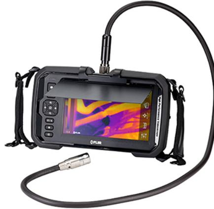
The FLIR VS80 series is a versatile, professional videoscope system that can be used to inspect locations that are difficult or unsafe to access.
